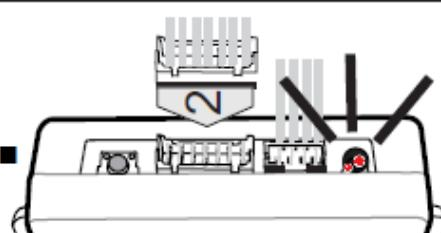
3. Plug the **connector 2** into the INT-SL+ interface.
