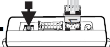
1. Press and hold the programming button. Plug in the **connector 1** in the INT-SL+ interface.
